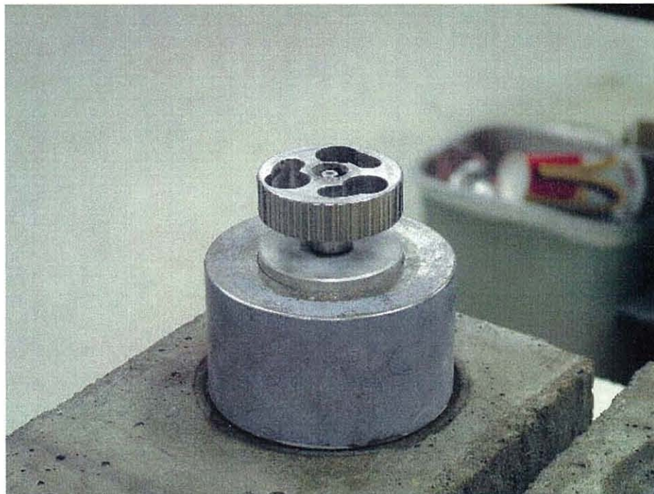
Figure 11 – Coupling Device and Counterpressure Ring for Direct Tension Test
