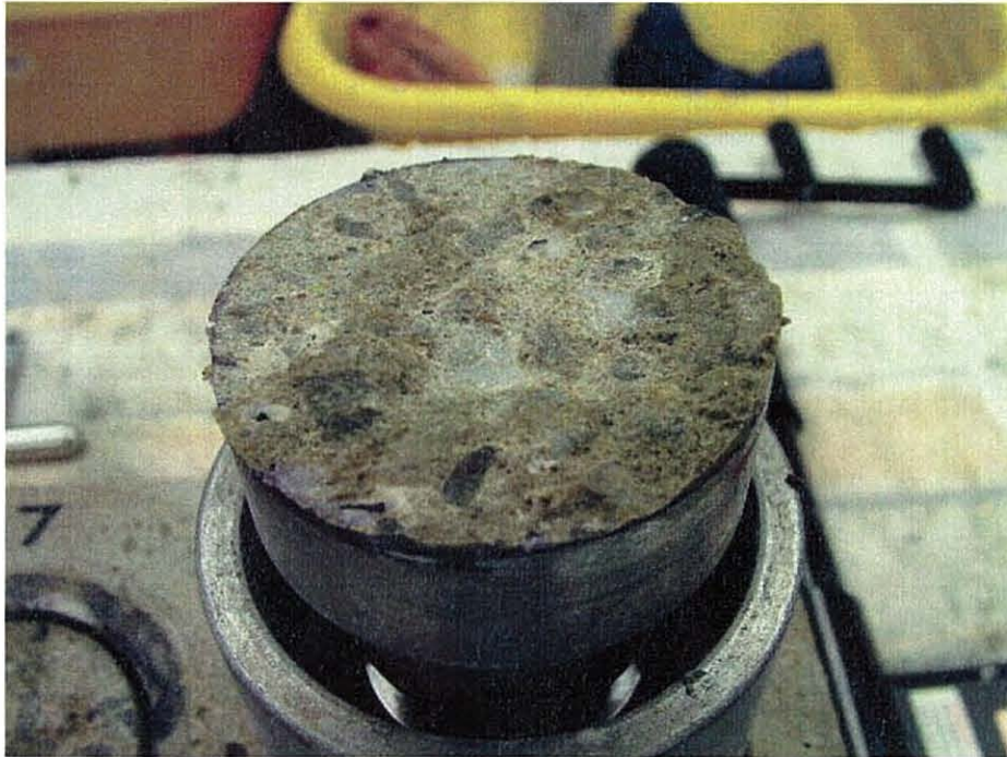
Figure 36 – Typical Surface Break with Direct Tension Test (View of Metal Disk)
