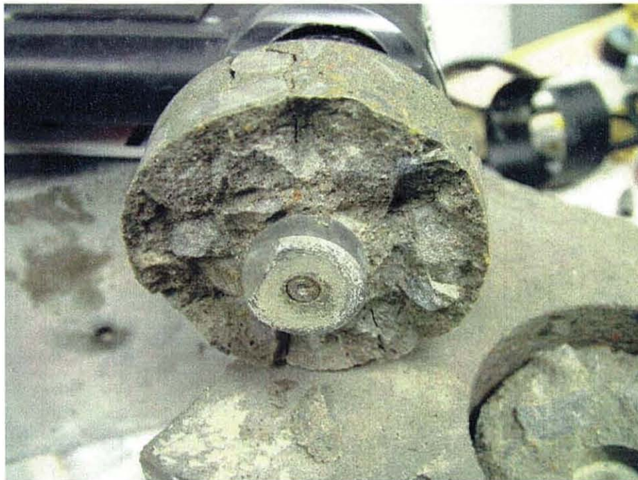
Figure 15 – Typical Failure Surface of Modified Pullout Test (Extracted Partial Core)
