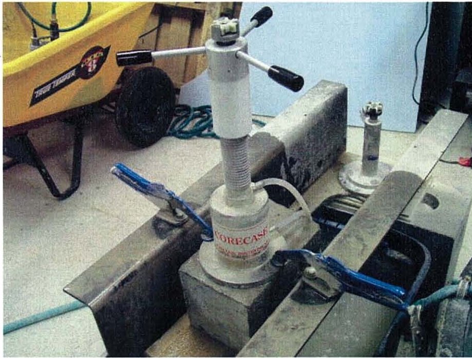
Figure 10 – Coring Equipment for Direct Tension and Modified Pullout Tests
