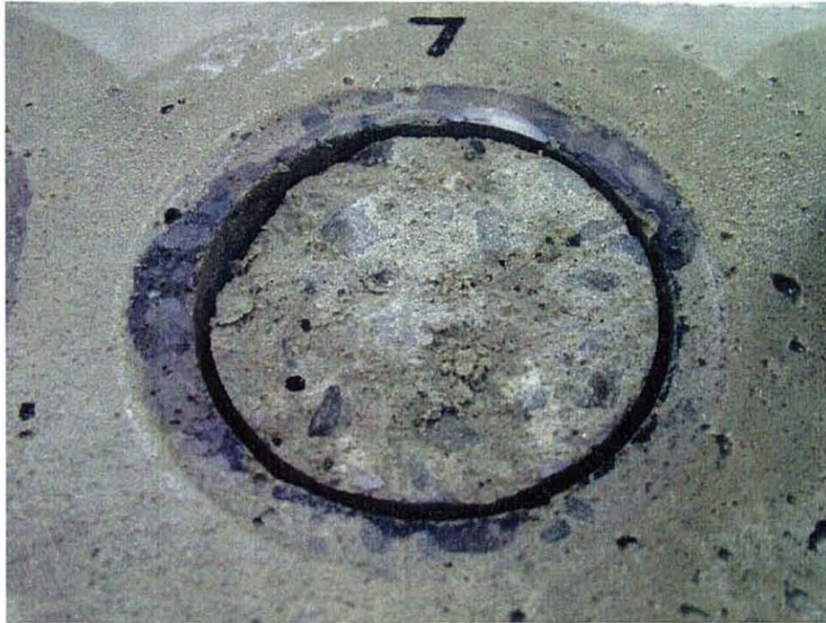
Figure 37 – Typical Surface Break with Direct Tension Test (View of Concrete Surface)
