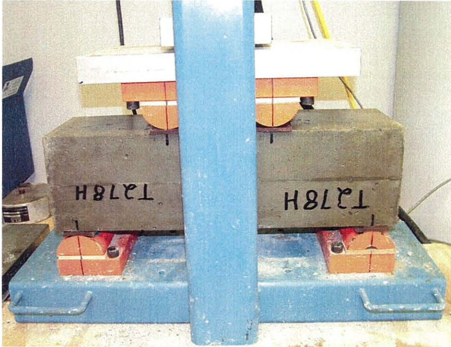
Figure 4 – Reaction Frame for Third-Point Flexural Beam Test (ASTM C78)
