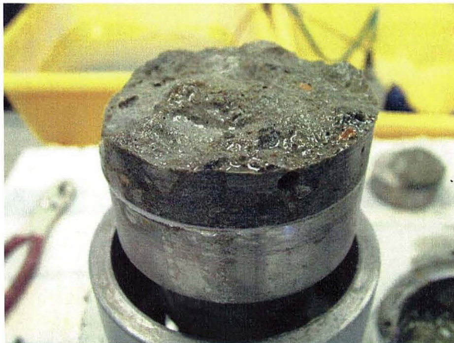
Figure 13 – Typical Failure Surface of Direct Tension Test (Extracted Partial Core)
