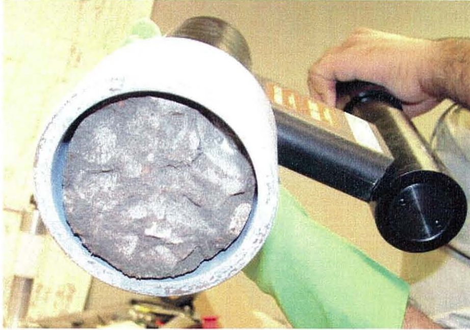
Figure 35 – Example of Coarse-Aggregate Pullout (Direct Tension Extracted Core)
