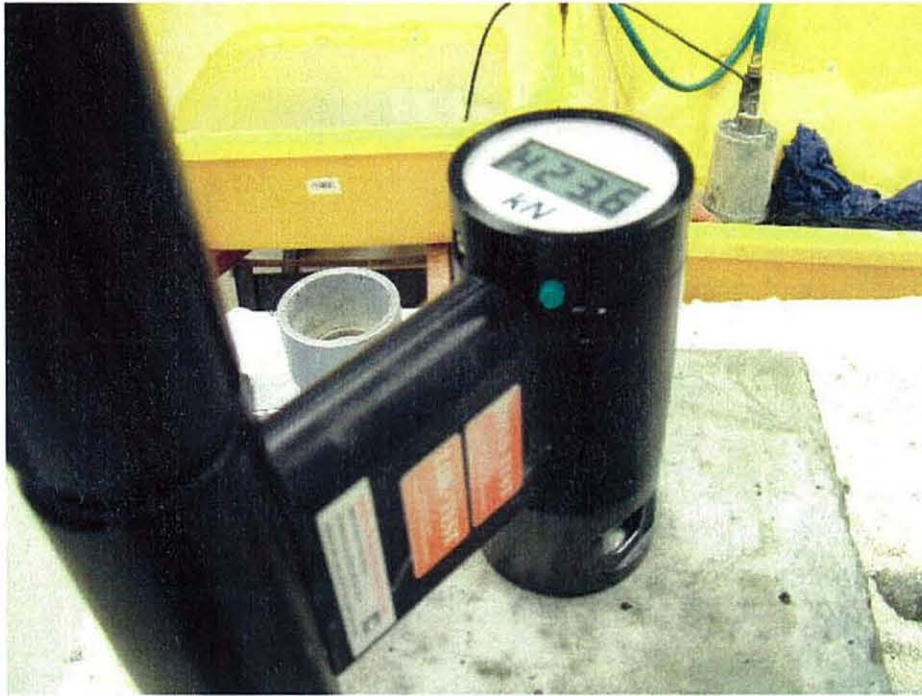
Figure 6 – Hydraulic Pull Machine for Pullout, Direct Tension, and Modified Pullout Tests
