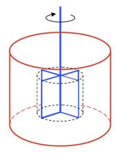
Fig. 2: The concentric cylinder geometry of the ICAR Plus
