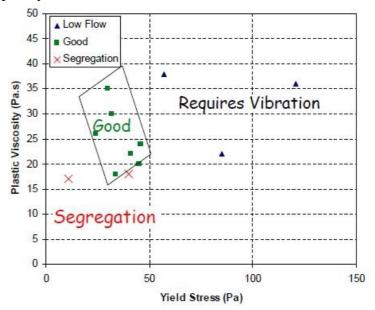
Fig. 8: Workability for self-compacting concrete
