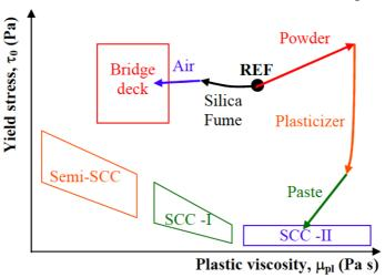
Fig. 10: Examples of how to steer concrete rheology into a specific target box
