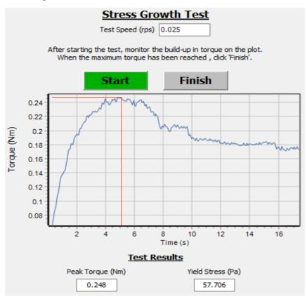
Fig. 4: Stress Growth Test
