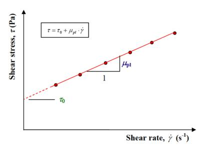
Fig. 7: Fundamental rheology parameters yield stress,  $\tau_0$  (Pa), and plastic viscosity,  $\mu_{pl}$  (Pa·s), for the Bingham model
