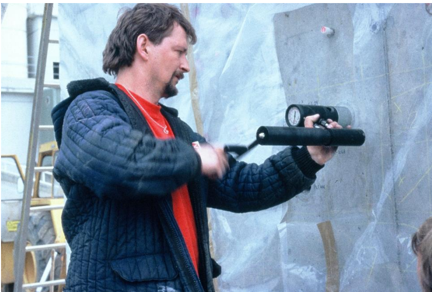
Fig.16. LOK/CAPO-Test in progress.
