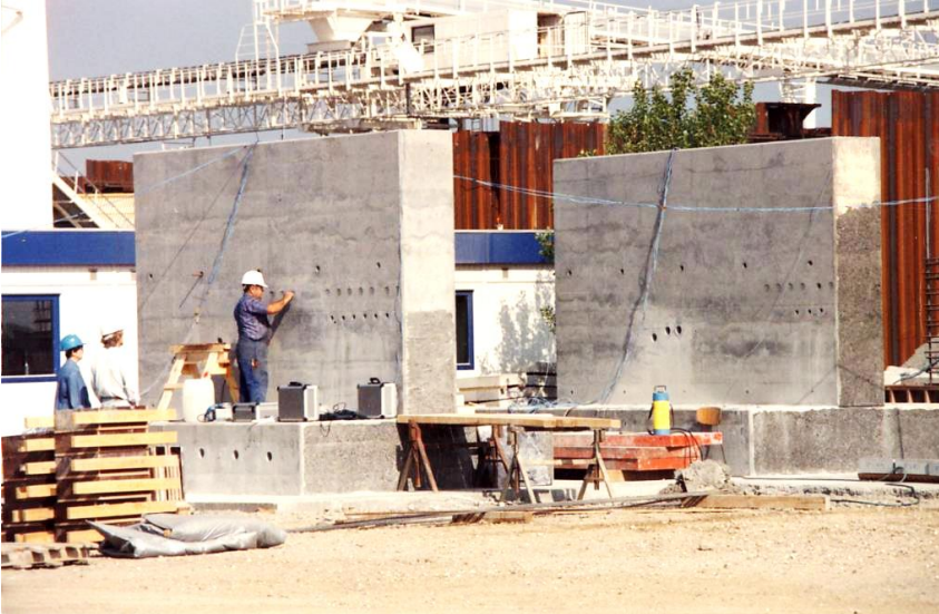
Fig.12. Trial casting, tested for chloride diffusion, strength and LOK-Test / CAPO-Test of the cover layer in relation to maturity to establish acceptable intervals.
