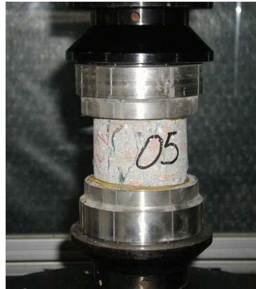
Fig. 14—Core being tested for compressive strength using “sand box” caps described in EN 12390-3.<sup>23</sup>
