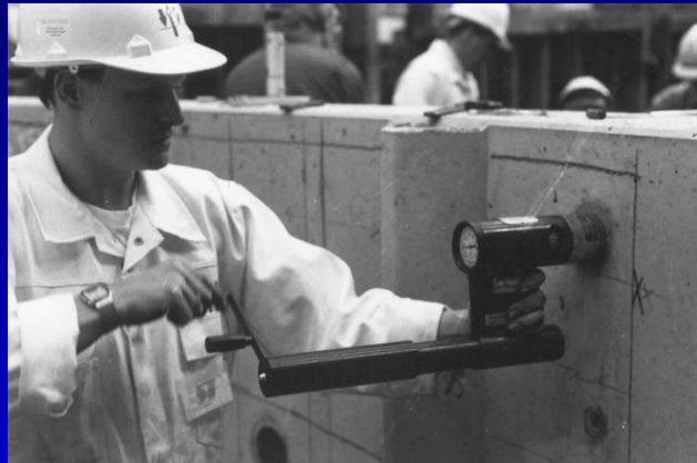
Translink, UK, Residual strength of tunnel segments
