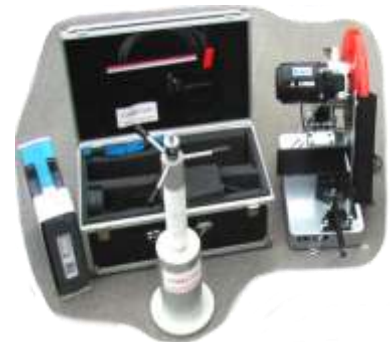
Figure 6 The drill machine and the CORECASE CEL-100 with coring rig and the diamond saw for producing the specimens.
