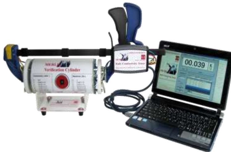
Figure 4 The MERLIN ® system shown with the verification cylinder.
