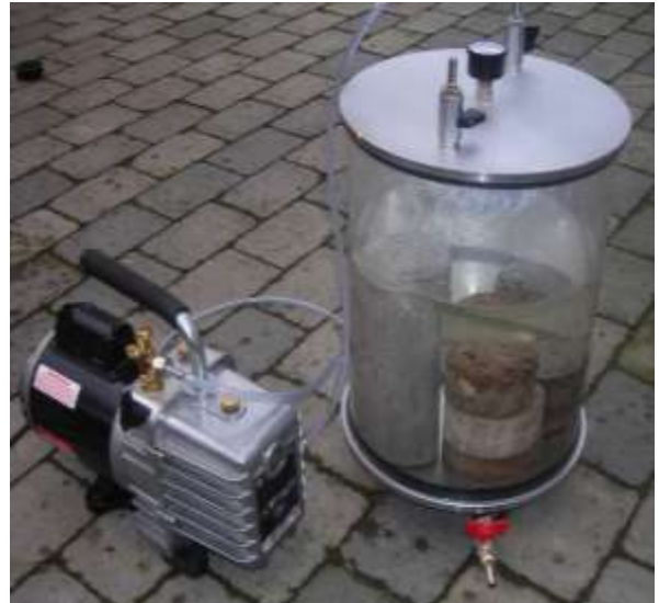
Figure 7 The PR-1070 Vacuum desiccator for saturating 16 specimens (dia. 100 mm x 50 mm) and the PR-1081 vacuum pump with hose with <10 mm Hg vacuum.
