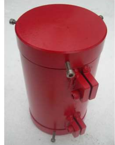
Figure 5 The precision steel mould for 100 mm in diameter, 200 mm high specimens.
