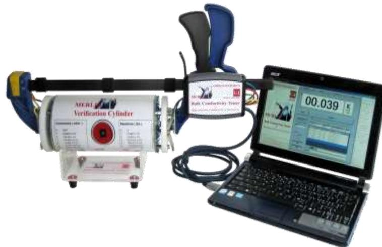
**Figure 4** The MERLIN® system shown with the verification cylinder.
