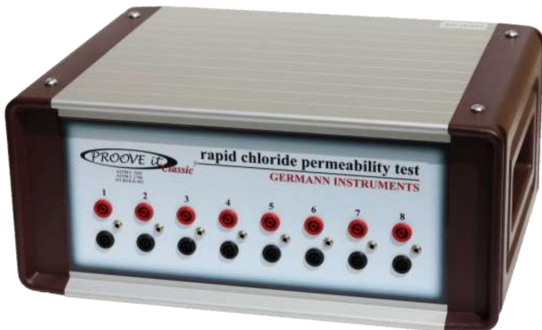
**Figure 1** The PR-1050 Proove'it Classic for up to 8 cells.
