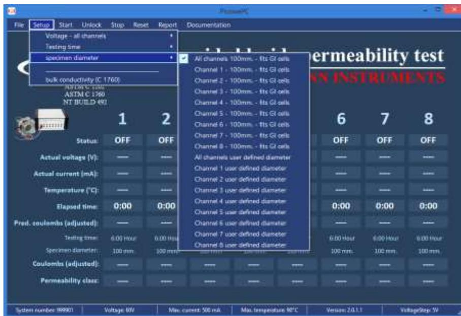
The default selected option is 100 mm diameter for all channels. For each sample the actual diameter has to be entered, enabling the software to calculate the correct Permeability Class according to the ASTM C 1202 classification system. The program will automatically apply the corrections to the ASTM standard’s 95 mm specimen size.
