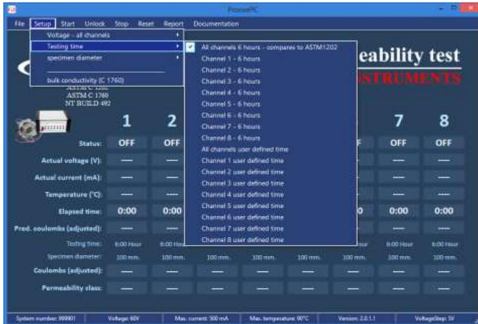
Testing time can be set whether to be the default 6-hours period (ASTM C 1202), or any other testing time (NT Build 492) for each channel.
