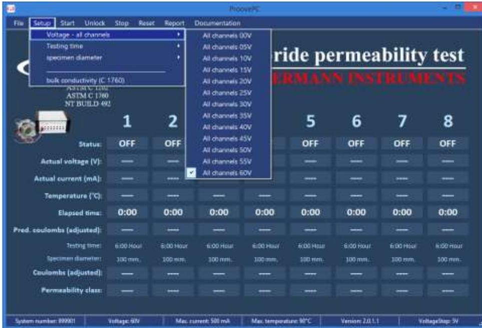
The ASTM C 1202 standard specifies the voltage to be at 60 V. For the NT BUILD 492 the start-up voltage is 30 V and, depending on the initial current measured, the final testing voltage and the time tested over are selected according to what is stated in the NT BUILD 492 standard requirements.
