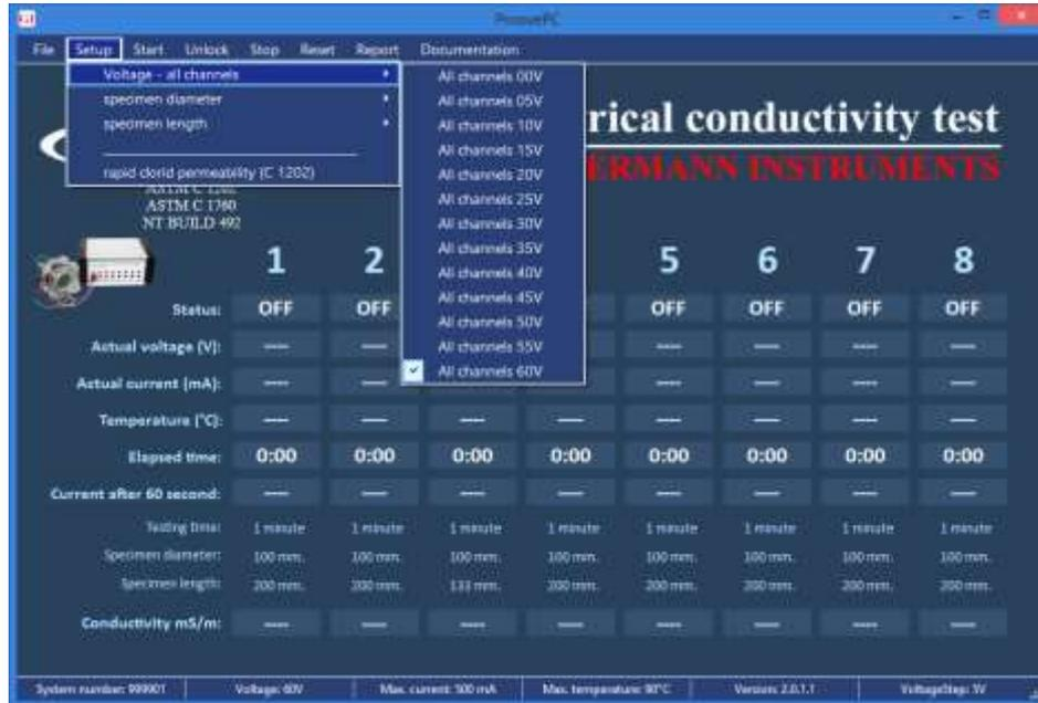
Select the testing voltage for the channels; however, the standard voltage according to ASTM C 1760 is 60 V.
