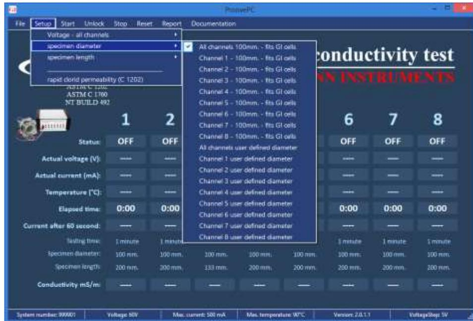
Select one of the default 100 mm diameter options from the menu or input the actual diameter for the desired channel.
