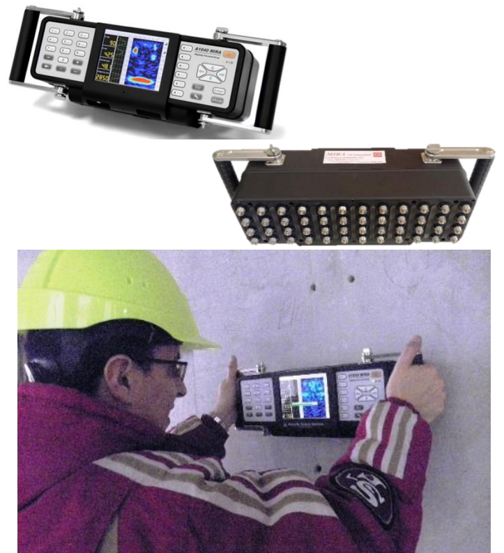
Figure 3. The MIRA ultrasonic-echo tomographer. To the left, front face displaying a cross section scan; to the right, the 4 x 12 transducer array antenna; and at the bottom, testing in progress.
