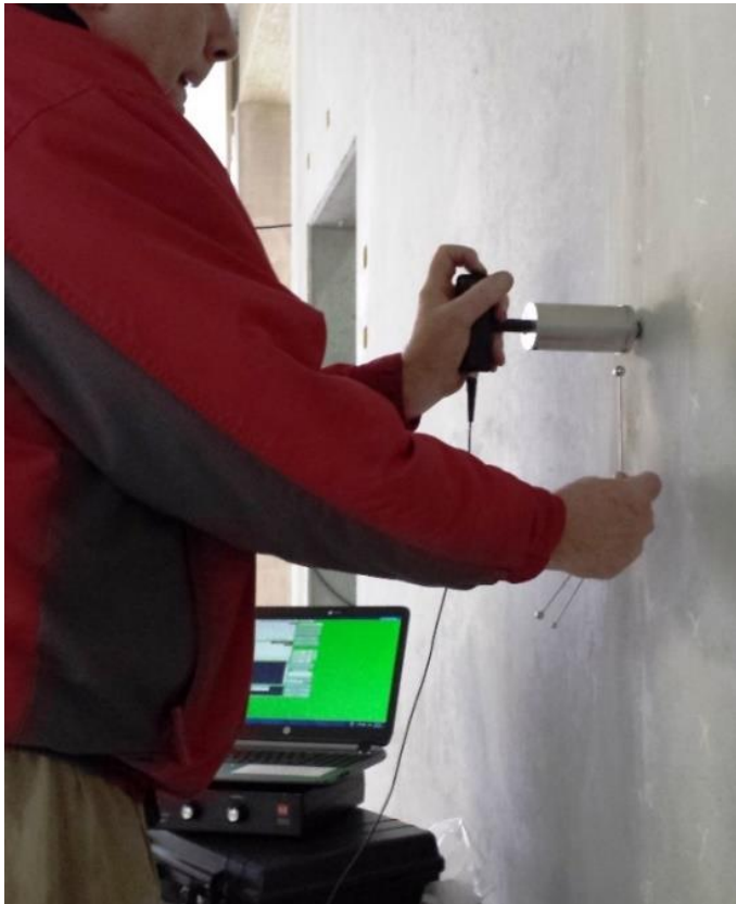
Figure 1. The Impact-Echo method.
