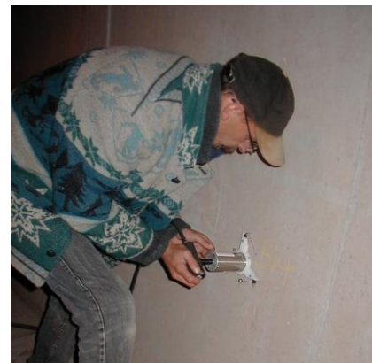
Tunnel lining thickness, Germany
