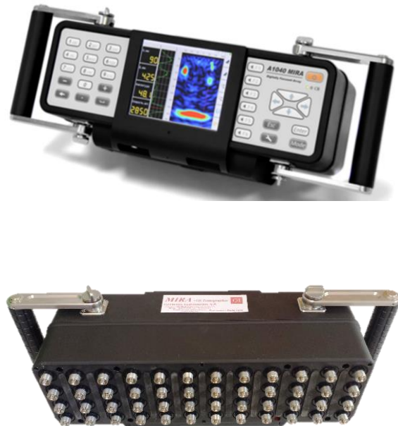
Figure 7. The ultrasonic-echo tomographer: (top) top face with display showing 2D cross section image; (bottom) the 4 \times 12 transducer array antenna.
