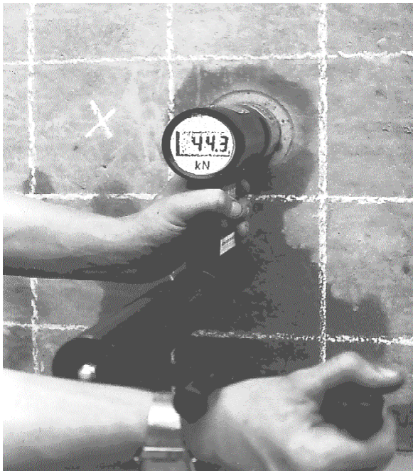
Figure 22: Loading of the Capo-Testing in progress.
