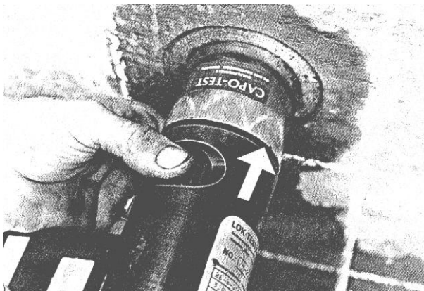
Figure 21: Coupling of the hydraulic pull machine.
