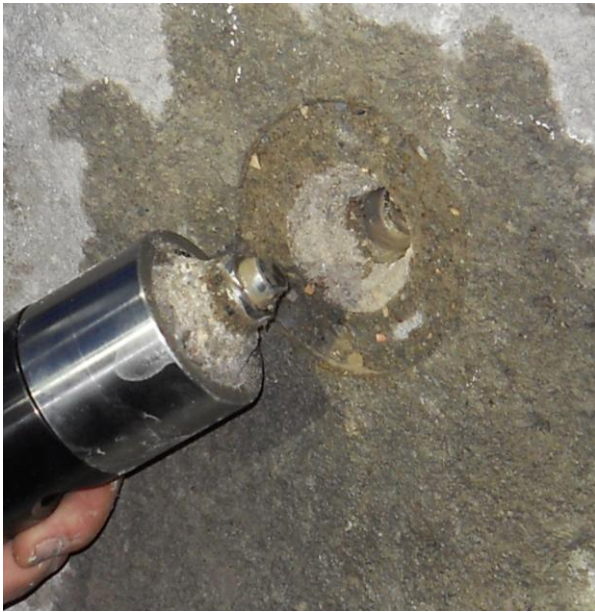
The completed CAPO-TEST. Notice the unfolded CAPO ring on the cone pull bolt.
