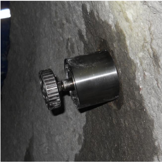
After fully expansion of the CAPO ring in the routed recess the counter pressure is installed on the surface and the coupling threaded to the center pull bolt
