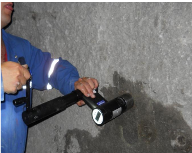
The hydraulic CAPO-TEST instrument is coupled to the coupling and the slack removed between instrument and counter pressure. Loading takes place by turning the instruments handle slowly.
