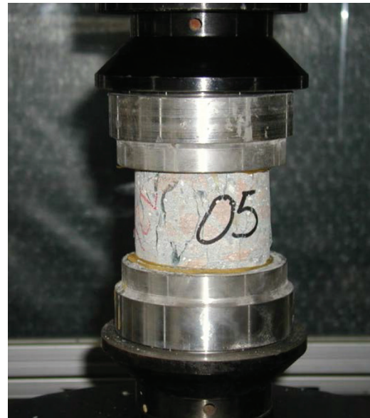
Fig. 14—Core being tested for compressive strength using “sand box” caps described in EN 12390-3. 23
