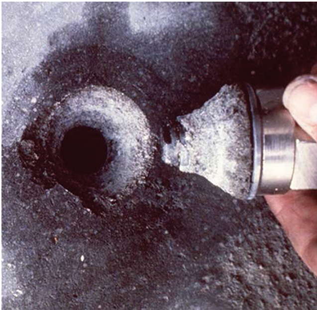
Fig. 4—Example of unacceptable CAPO-TEST; surface was not flat and a complete ring was not formed at surface.
