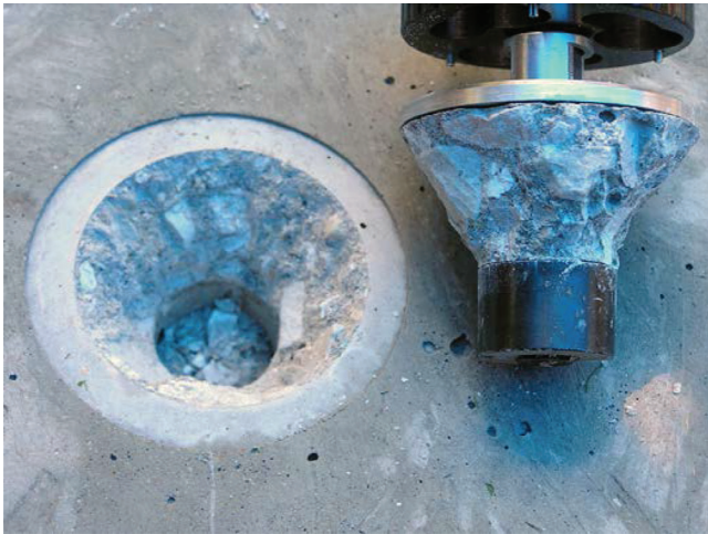
Fig. 11—Dislodged conical fragment from LOK-TEST, with debris at bottom of hole due to multiple microcracks within compression band.
