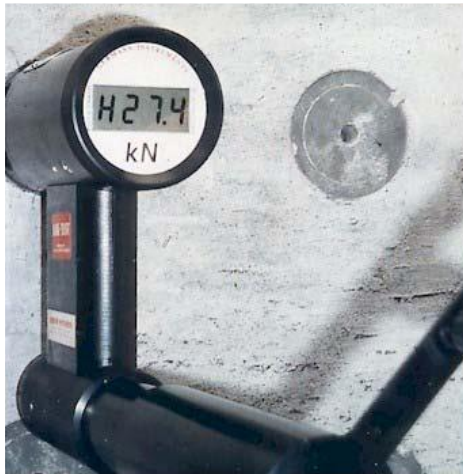
LOK-TEST being performed on a wall for quality control of the finished structure. “H” on the display shows the highest pullout force. The L-40 Insert is used.
