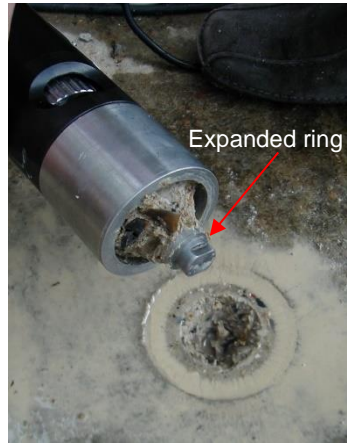
View of valid CAPO-TEST of a slab. Note the well-formed failure ring on the surface of the slab.
