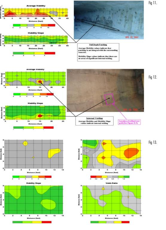
fied and quantified deficiencies such as incomplete consolidation of concrete and honeycombs, debonded repair patches, and incompletely filled areas of voids.
