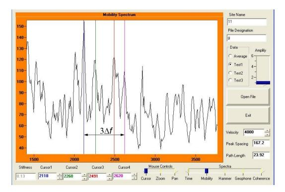
Fig. 7. The mobility plot registered by the Impulse Response method for the pile no. 11.
