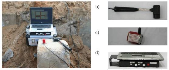
Fig. 3. The view of the : a) impulse response equipment: b) hammer, c) geophone, d) amplifier
