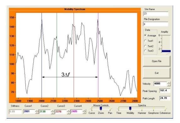
Fig. 8. The mobility plot registered by the Impulse Response method for the pile no. 23.
