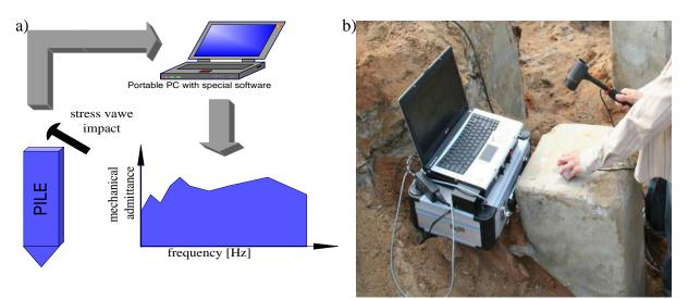
Fig. 2. Impulse Response test method: a) the concept, b) example of using in practice
