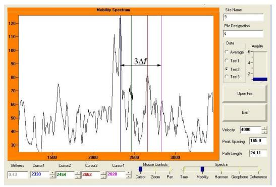
Fig. 6. The mobility plot registered by the Impulse Response method for the pile no. 9.
