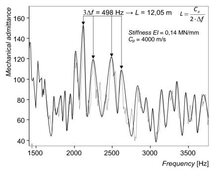
Fig. 5. The visual mobility chart with marked parameters to determine the length of concrete prefabricated piles
