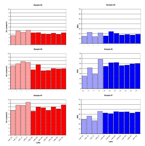
Figure 7: Graphical presentation of the air content and specific surface area (SSA) of the 3 samples analysed. Hatched: manual readings, solid: automatic analysis
