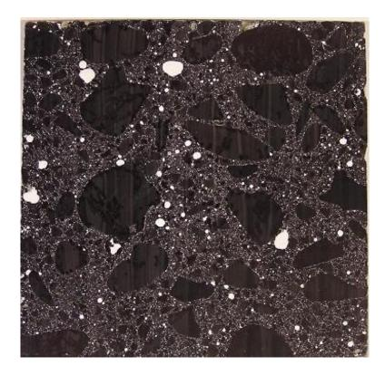
Figure 3: Appearance of sample #5 after being coloured black and white  $BaSO_4$  powder filled into the air voids.
