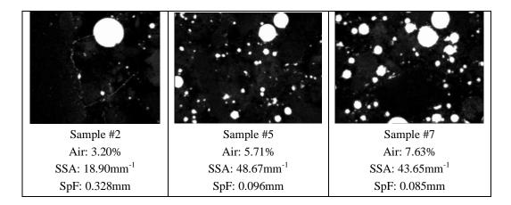
Figure 6: Close-up of the air void structures of the samples analysed. The images were collected during analysis. The average results of the automatic analysis are provided below the images (from Tables 2, 3 & 4). Abbreviations: SSA: specific surface area, SpF: spacing factor
