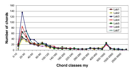
Figure 8: RapidAir chord length distribution determined by 7 laboratories.
