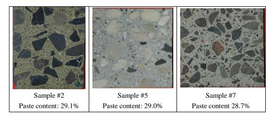
Figure 1: Appearance of the lapped samples. The manually determined paste content of the samples is noted below the images.
