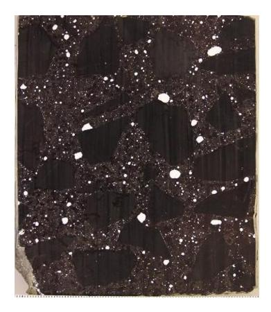
Figure 2: Appearance of sample #2 after being coloured black and white BaSO<sub>4</sub> powder filled into the air voids.
