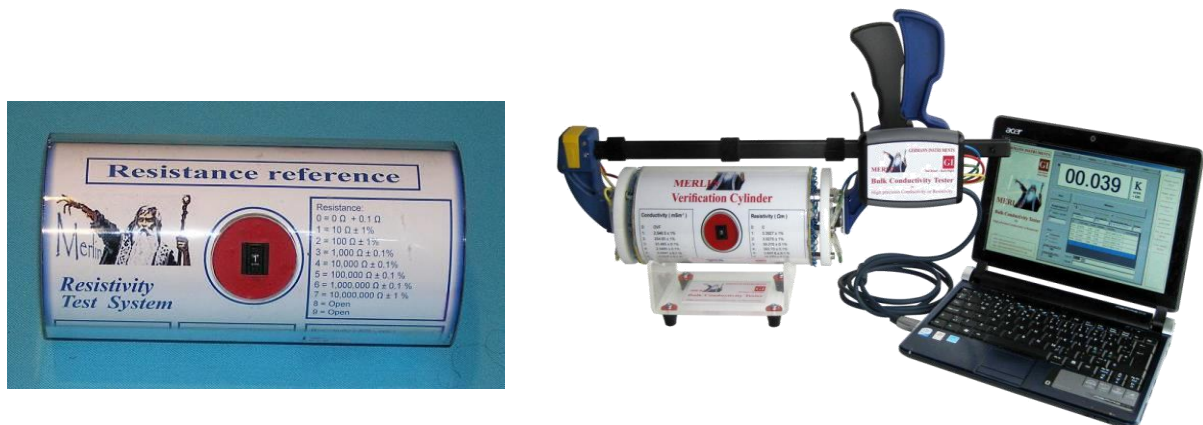
Fig. 12. The verification cylinder is used to make sure the system is working properly before performing a measurement.
