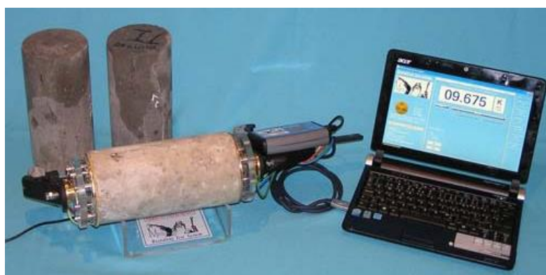
Fig. 10. Merlin being used on a water-saturated cylinder. A conductivity of 9.675 mS/m is measured after 2 seconds, the usual time taken to obtain a stable reading.
