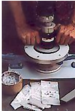
Fig.1. Laboratory testing. Profile grinding of specimen subjected to 35 days of immersion in the laboratory. Chloride content of each sample is determined using the RCT. The profile obtained is shown in the right figure. An apparent chloride diffusion coefficient of 29 \text{ mm}^2/\text{y} is estimated by fitting the solution Fick's Second Law of Diffusion in accordance with ASTM C 1556 or NT BUILD 443
