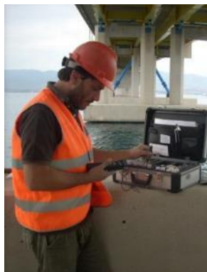
Fig.2. On-site testing. Profile grinding in progress on a sea structure (left) and chlorides being measured with the RCT (middle) after each step of grinding. From the profile (red dots in the right figure, neglecting the values of the first 5 mm affected by carbonation) an apparent diffusion coefficient of 10.9 \text{ mm}^2/\text{y} is estimated. For the cover layer of 80 mm and for a critical threshold chloride value to initiate corrosion of reinforcement of 0.05% Cl/concrete mass, the estimated remaining service life is 78 years. Similarly, for C_{cr} = 0.10\% Cl/concrete mass, the estimated remaining service life is 111 years, all other factors being constant.
