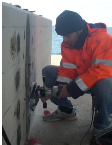
Fig.2. On-site testing. Profile grinding in progress on a sea structure (left) and chlorides being measured with the RCT (middle) after each step of grinding. From the profile (red dots in the right figure, neglecting the values of the first 5 mm affected by carbonation) an apparent diffusion coefficient of 10.9 \text{ mm}^2/\text{y} is estimated. For the cover layer of 80 mm and for a critical threshold chloride value to initiate corrosion of reinforcement of 0.05% Cl/concrete mass, the estimated remaining service life is 78 years. Similarly, for C_{cr} = 0.10\% Cl/concrete mass, the estimated remaining service life is 111 years, all other factors being constant.
