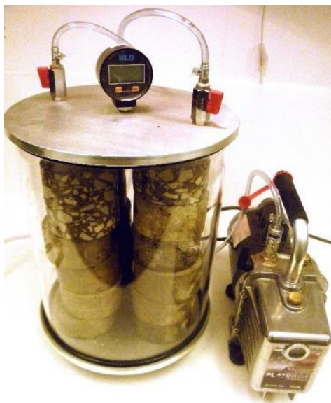
Fig. 3. The PR-1070 Vacuum desiccator for saturating max. 24 specimens (dia. 100 mm x 50 mm) and the PR-1081 vacuum pump with hose, <10 mm Hg vacuum.
