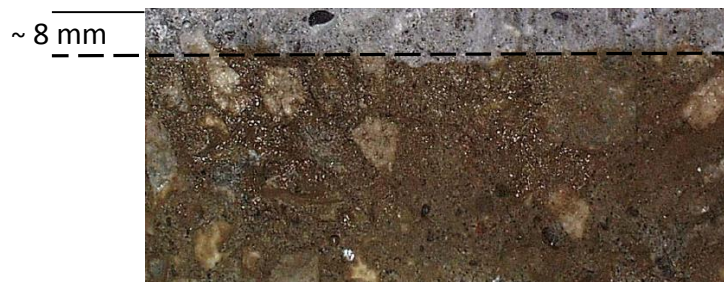
Fig. 6. Chloride penetration depth of ~8 mm on a specimen after NT BUILD 492 testing
