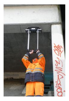
Fig. 1. The extension handle mounted the MIRA antenna
