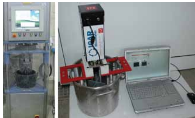
Figure 2. Rheometers, ConTec Viscometer 5 (left), ICAR Rheometer (right)
