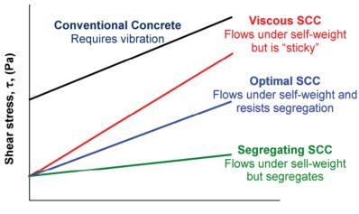
Shear strain rate,  $\dot{\gamma}$ , (1/s)
