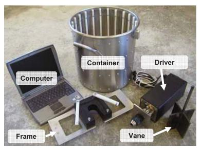
vane has a diameter and a height of 127 mm.
