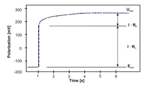
Fig. 1. Typical polarisation pattern
