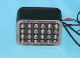
The averaged signal recorded by the receiving transducers is stored in the hand-held unit as a time-domain waveform. An example of such a waveform is shown at the top of the next page. In this case, the test was done on a solid concrete slab with a thickness of about 200 mm. The figure on the left side of the next page shows signal amplitude as a function of time (A-Scan). The three peaks are due to multiple reflections
