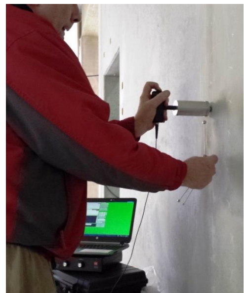
Fig. 2. DOcter Impact-Echo in progress.
