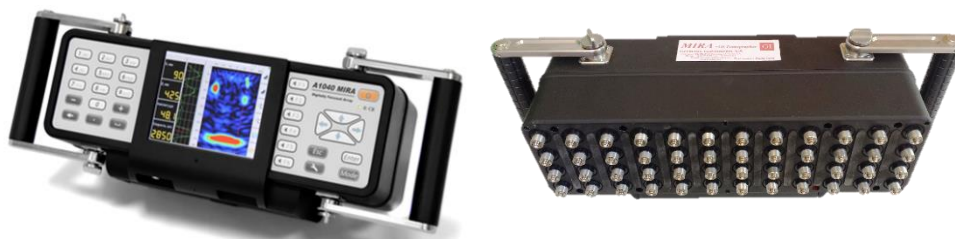
Fig. 3. The MIRA ultrasonic-echo tomographer. Front face at the left with the display showing a cross section scan. To the right, the 4 x 12 transducer array antenna.
